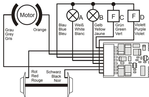
If the bulbs for the directional headlights are floating (isolated against wheel pick up and chassis) and connected according to above figure, they will shine brighter
